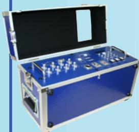
This is to receive and record tag ID. There are 2 types of receiver; 5ch and 8ch. 4m width mat is applied to 5ch, on the other hand, more than 4m are applied to 8ch. Both type of receiver run on DC12V power or a car battery. The max power consumption is 4A.
